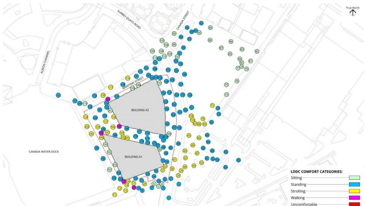
Image above: Configuration 1: Proposed Development with existing surrounding buildings and proposed landscaping, ground level, windiest season.
